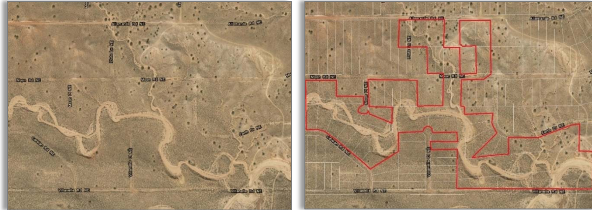
Figure 3 - These two images show the impacts of the existing subdivision of seemingly vacant land that complicated ROW acquisition. The red outline identifies the parcels that would need to be acquired to capture the arroyo.
